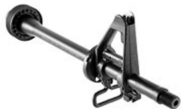
length gas tube (available separately) Available as Stripped or complete Barrel Assembly This Brownells Retro A1 rifle barrel is machined from ultra-strong 4150 chrome-moly steel, and is magnetic particle inspected when finished to ensure there are no hidden flaws that could shorten its service life.
