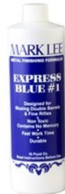
No damp cabinets or long rusting periods required to get top-quality, good-looking blues and browns. Heat gun or part to 150°-200° F. with propane torch; swab on solution, and card with soft wire wheel or fine steel wool. Blue #1 does require parts be immersed in boiling water for 5 minutes before carding.
